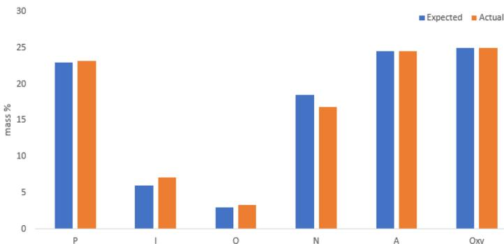
Fig 7. Expected and actual values of hydrocarbon groups ASTM standard (mass%)
