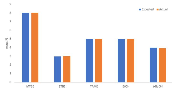
Fig 8. Expected and actual values of individual components ASTM standard (mass%)
