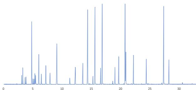
Fig 3. Separation of PIONA calibration standard
