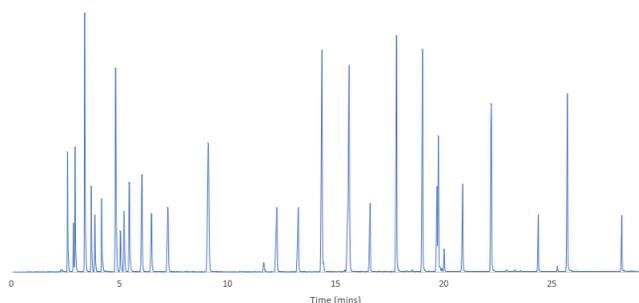
Fig 2. Separation of ASTM D8071 calibration standard
